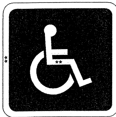
Figure 38-19. International Symbol-of-Accessibility Parking Space Marking with Blue Background and White Border Options
