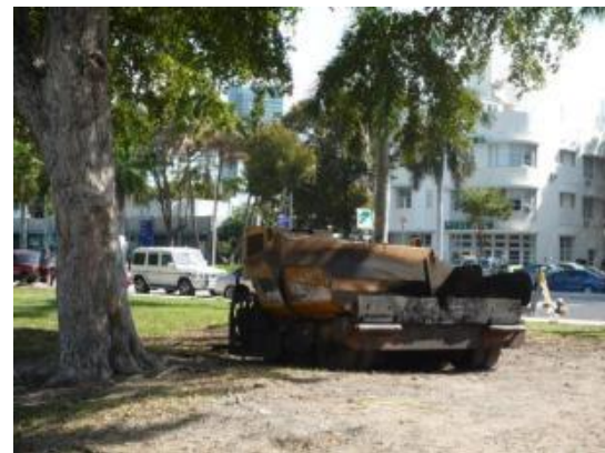
Figure 5.2.4.1-8. Do not place heavy equipment in root zone.
