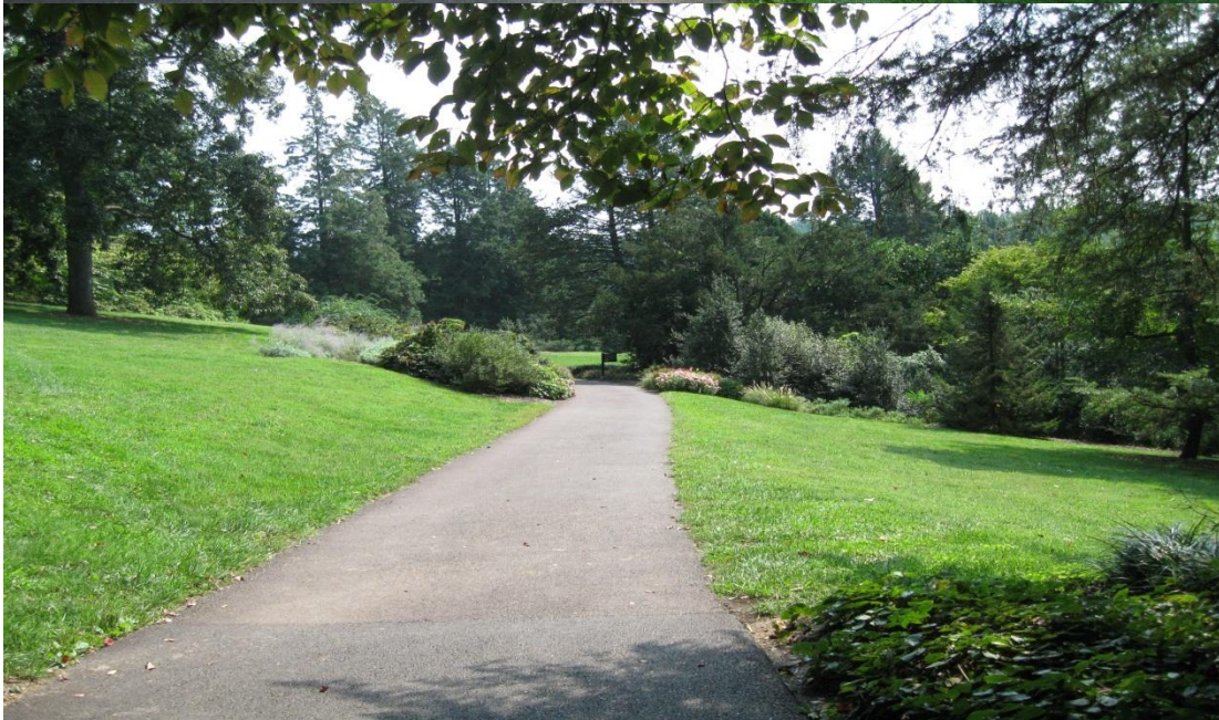
Figures 5.3.10-4a and b. Paths can be disconnected by sheet flowing onto a vegetated area of an adequate size and slope.
