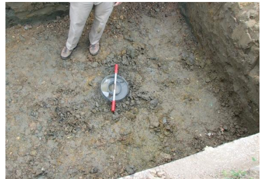
Figure C-2. Double-ring infiltrometer test.
