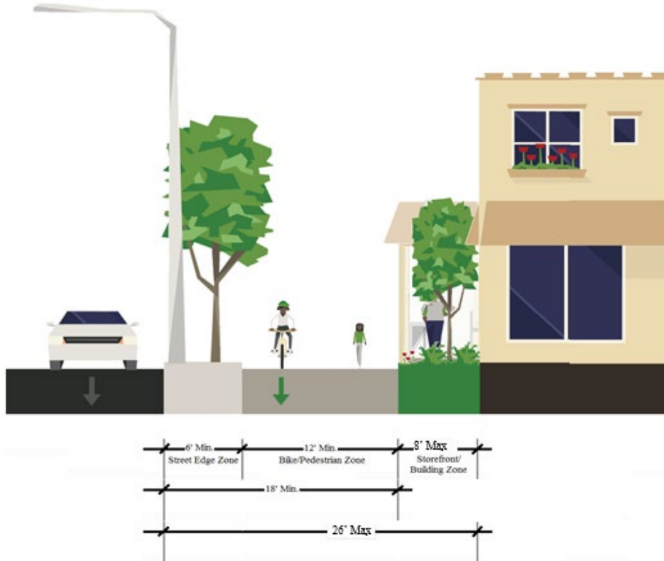
Figure 4. Diagram of Street Edge, Bike/Pedestrian, & Storefront/Building Zones
