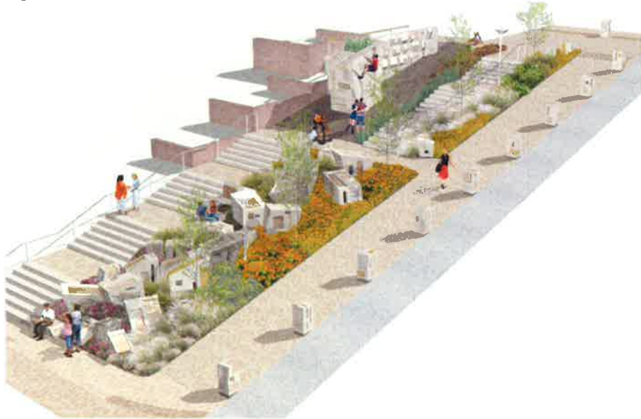
A perspectival rendering, detail from the Design Development package, depicting the eastern portion of the Scramble at the eastern half of the 100 East block of 1st Street (this rendering shows some of the streetscaping features that were not pursued into CDs and the climbing wall that was removed during the value engineering process)
