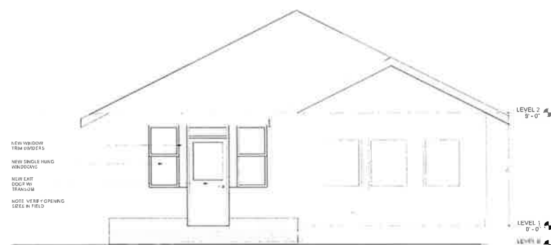
1 NORTH ELEVATION (W/O RAMP) 3/8" = 1'-0"
