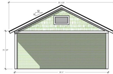
1 Carport Front Elevation Scale: 1/8"
